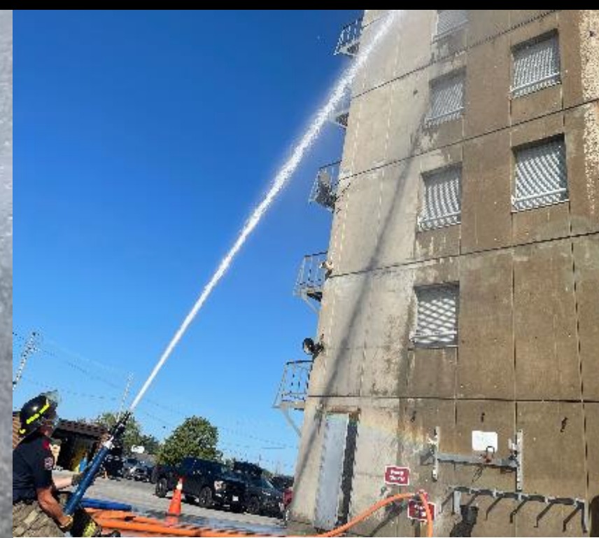
Opened fully 1003Lpm (264 gpm) Take nozzle reaction to ground
